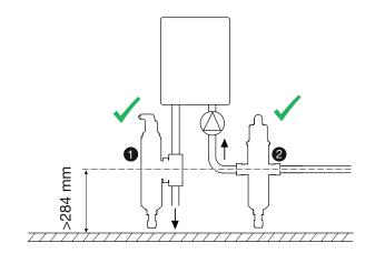
A dirty, problematic system would benefit from installing the combined unit in the return pipe, as close to the boiler as practically possible, or after the last tee connection in the return line. The small waterways in boilers do need consideration depending on system circumstances.
